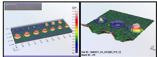
**Figure 5.** Shows detailed topography images of a missing deposit. The smaller deposits in the image on the left are 3-10 mils from left to right. In the zoomed image on the right, 6, 7, and 8 mil deposits are shown.
